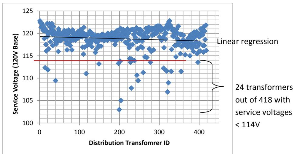
**Figure 2 - Lowest service voltage for each distribution transformer/secondary**
