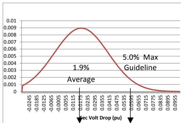
**Figure 1 - Distribution transformer/secondary max voltage drops**
